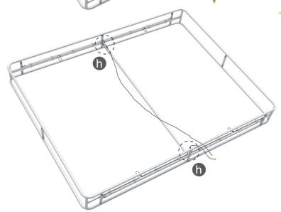
③ Connect those 2 adjacent LED light bars connected with Y-shaped connection wire, slightly adjust space between each LED light bar from 1" to 4".
