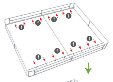
① Slide clips from LED light bars to align at holes of poles & press into.
